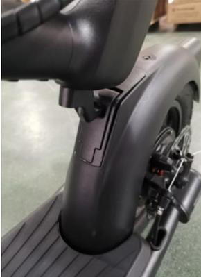
Then put the hook into the fixing seat hole.
