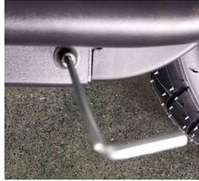
Insert a #4mm diameter wrench into the screw head. Turn the wrench counterclockwise.
