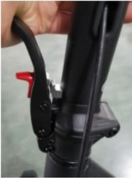
Pull the trigger back onto the pole.
