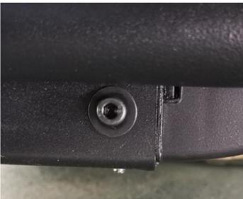
Locked: Put the pedal on and press it flat, insert the wrench into the screw head, and then turn it clockwise until it is locked.
