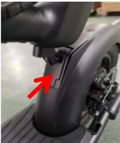
Press down on the hook holder, and then release the hook.
